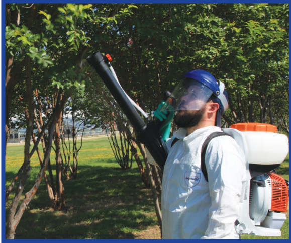
Figure 4. Backpack mist blower being used by a pest-control company employee to treat mosquito resting sites with a long-lasting insecticide. Source: Mike Merchant
